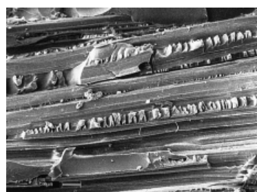
Figure 5 The fracture surface of 8-h-alkali-treated jute/vinylester composite showing strong bonding at the fiber/matrix interface (three point bend test).
